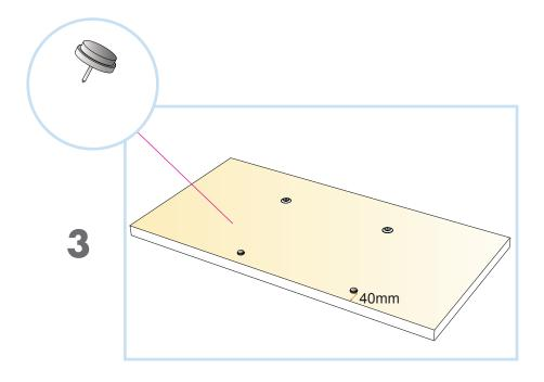
Wall spacers are used to maintain a consistent gap between the wall and the panel.
