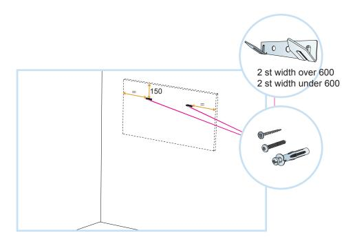
Please use appropriate screw fixings - not included. Two Connect One Hook fixings to be used for 600x600 square, 1200x600, 1200x300 rectangle. Attach the fixings to the wall as per the above image.
