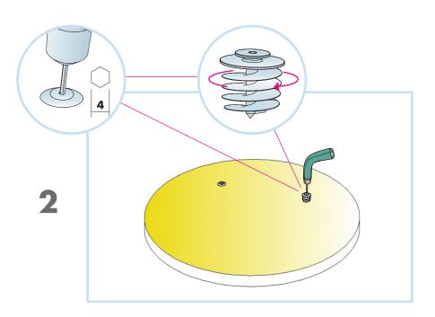
Using a hex attachment on a drill or an allen key, screw the absorber anchor into your marked area from previous diagram 1.
