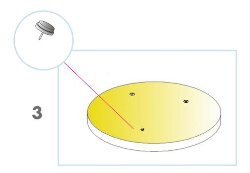
Wall Spacers are used to keep the gap between the panel and the wall even. Press into the panel around 100mm up from the lowest point.
