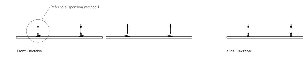
Note: Suspension Method 2 could also be used to hang these panels, reducing the number of hangers required.
