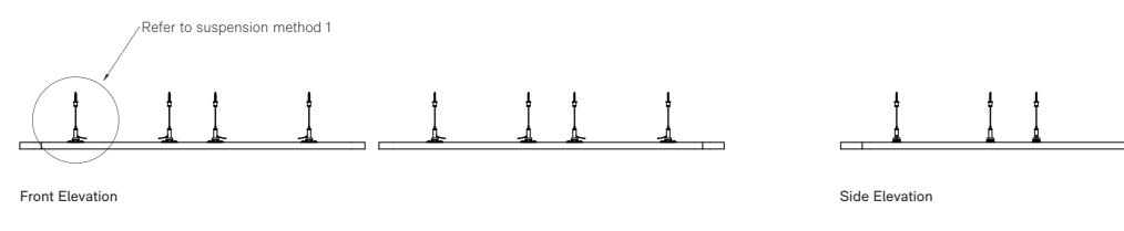
Note: Suspension Method 2 could also be used to hang these panels, reducing the number of hangers required.
