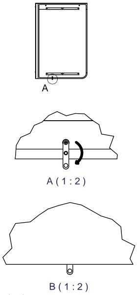
**Important**: Always use the bracket to fix the product to the wall. Use suitable screw for the actual wall type (not included)
