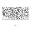
Fix using M6 or ø 4.5 mm c/sunk screw
