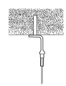
Position eyelet over drilled hole
