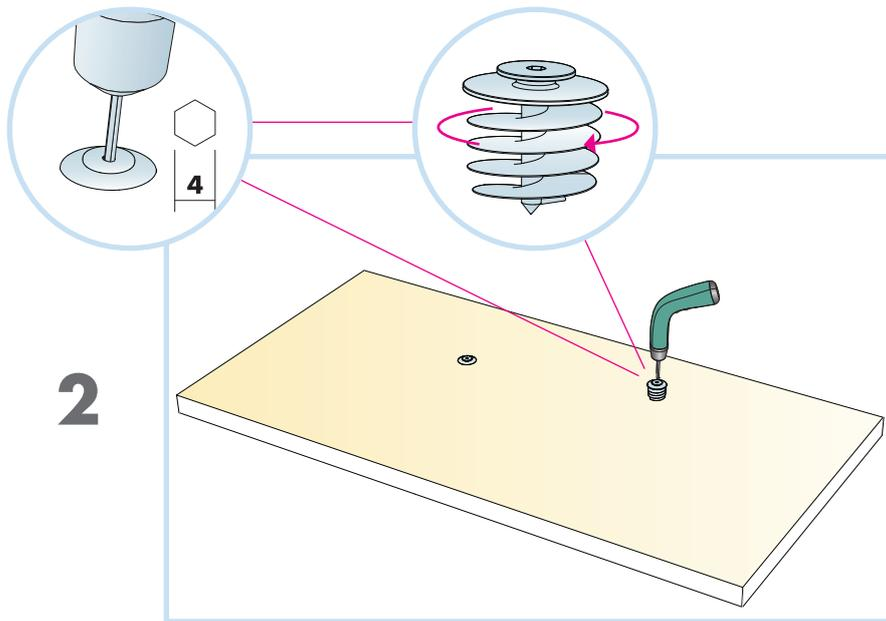
Using a screwdriver, screw the absorber anchor into your marked area from previous diagram 1b.
