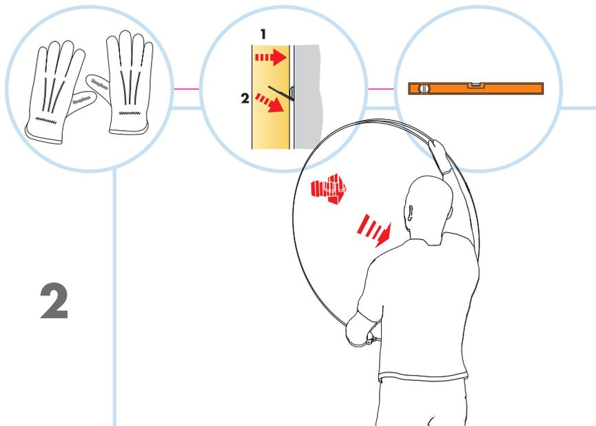
Carefully push the tile onto the One Hook fixings which are now fixed to the wall. Use gloves provided to handle the tile.
