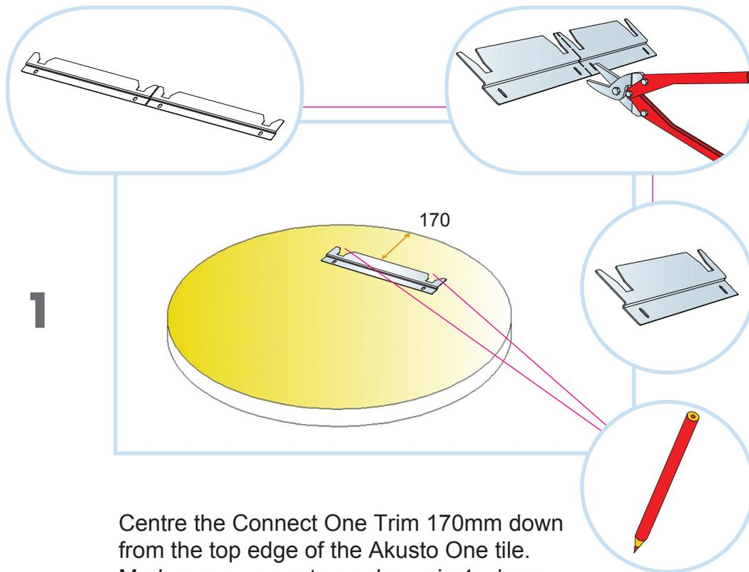
Centre the Connect One Trim 170mm down from the top edge of the Akusto One tile. Mark measurements as shown in 1 where the anchors will be placed.
