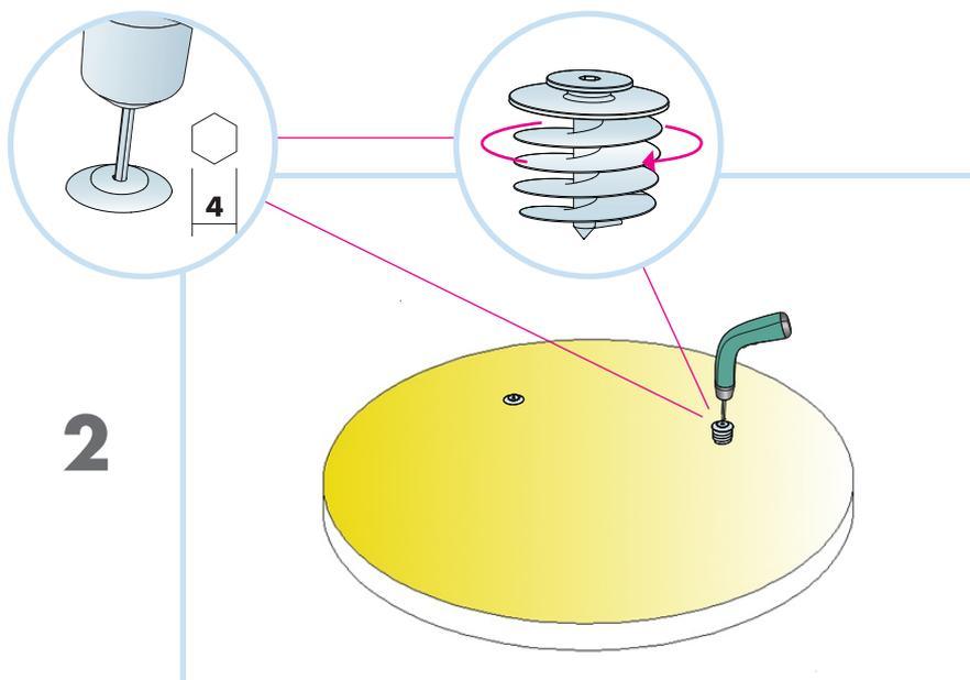
Using a hex attachment on a drill or an allen key, screw the absorber anchor into your marked area from previous diagram 1.
