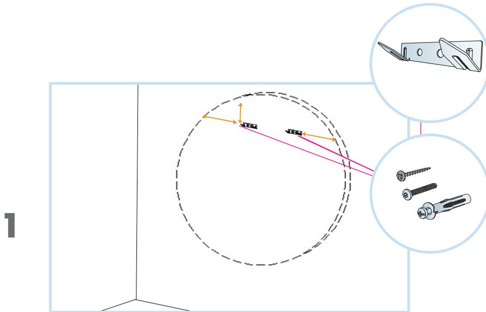
Fix hook fixings to wall. Please use appropriate screw/wall fixings - not included. Two Connect One Hook fixings to be used for 600 and 800 circle.
