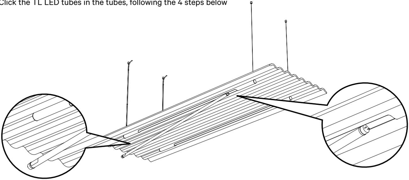
7 Slide the light diagonally into the LED tube
