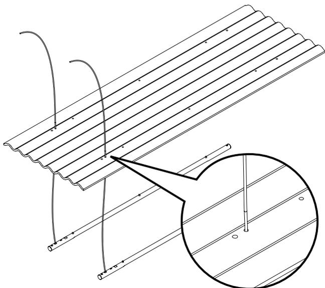
2 Mount lighttubes on the panel with the screws
