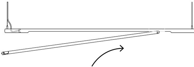
8 Slide the light horizontally as far as possible into the tube
